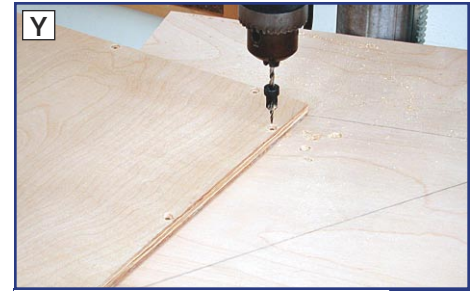
Countersinking Screw Holes
