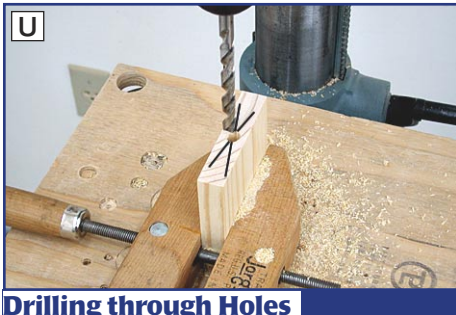
Drilling through Holes
