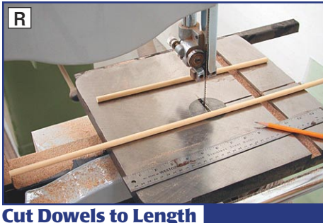
Cut Dowels to Length
